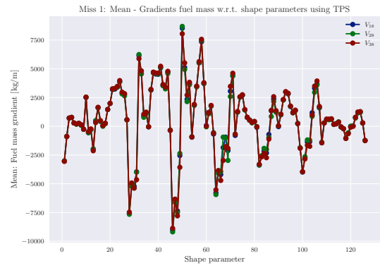
Figure 3.68: Total fuel mass gradients w.r.t. shape parameters, All versions, Mission 1, TPS
