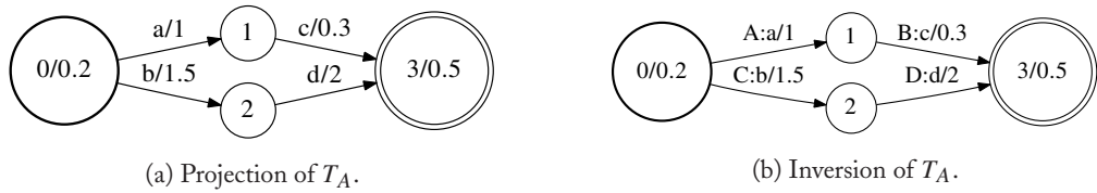
Figure 3.7: Examples of projection and inversion
