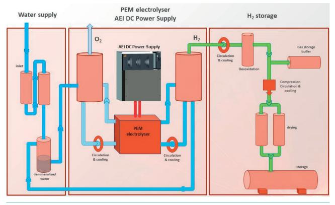
Figure 2. Block diagram of a typical electrolyser.
