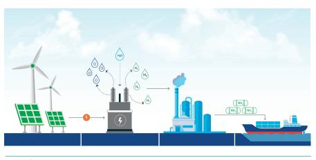
Figure 2. The green hydrogen and ammonia process.
