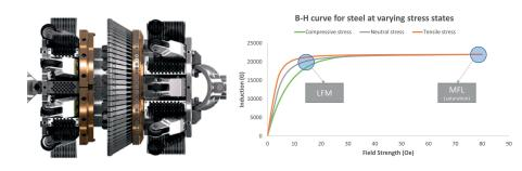
Figure 4. LFM dataset. LFM sensor array (left); B-H curve for steel (right).
