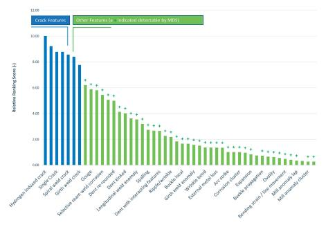
Figure 1. Critical anomalies for hydrogen – SME pairwise ranking.<sup>3</sup>
