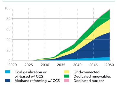
**Figure 3.** Global production of hydrogen derivatives as an energy carrier, by production route (million tpy hydrogen).
