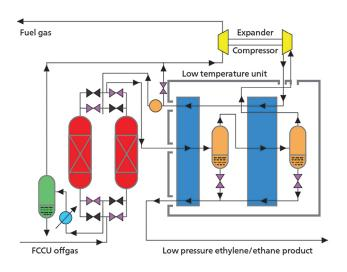
**Figure 2.** Ethylene treatment, distillation and recovery (source: Tomlinson 2002).
