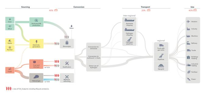
Figure 1. Hydrogen production and use flows in 2050 (the thickness of the flow lines approximates the volume of each flow indicating major production routes and end uses in 2050). Source: DNV 'Hydrogen Forecast to 2050'.
