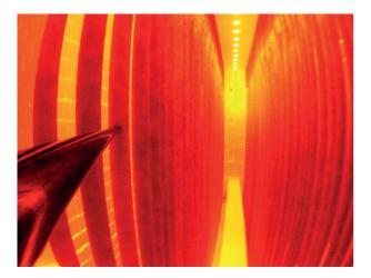
**Figure 4.** A thermal image taken whilst AMETEK Land's specialist engineer took a Gold Cup measurement.
