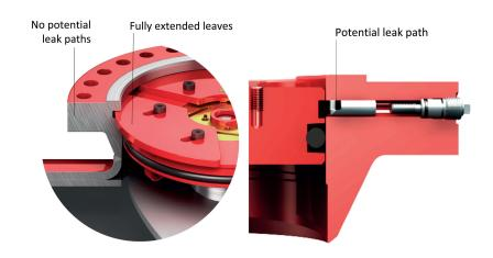
**Figure 6.** The new design of HT&P completion plugs. New completion plug set in place with extended leaves that fit in the flange groove; no leak paths (left). The old design of plug is held in place with segments that are extended with a screw mechanism drilled through the flange (right).
